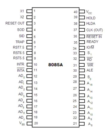
8085 is a 40 pin IC, The signals from the pins can be grouped as follows
